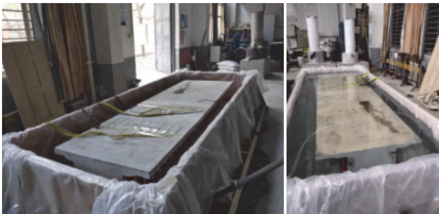
Figure 4. Girder corrosion test setup
