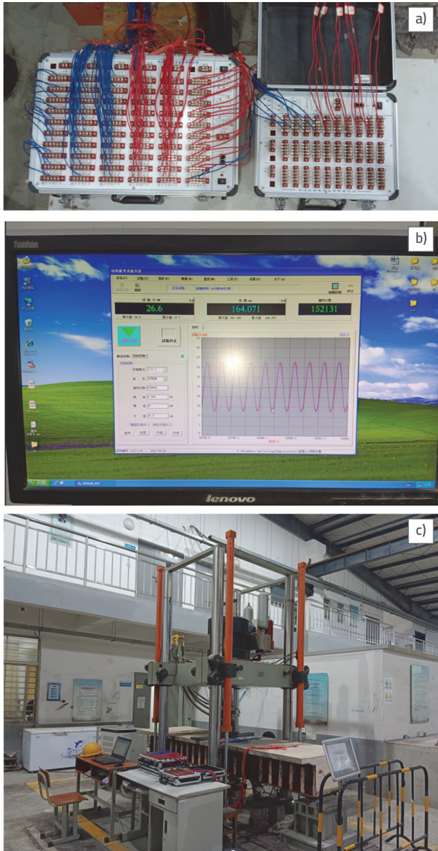
Figure 5. Girder fatigue test: a) Stress-strain sampling system, b) Fatigue loading system, c) Test girder loading
