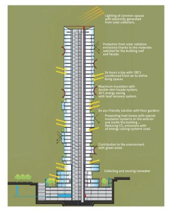
Figure 2. Energy-efficient features of building (modified image [31])
