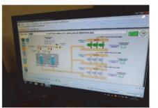
Figure 10. Building control centre automation system
